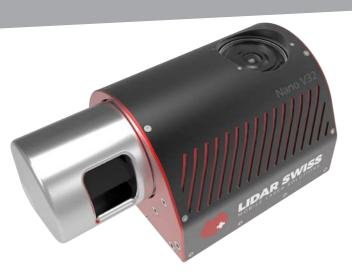
LS Nano V32 is a mini Lidar system specially designed to meet the market need for Multi-copters. Consists of Velodyne HDL-32E scanner, a 20mp mini camera, a suitable POS system and LidarsSwiss proprietary control unit, this 2.7kg Lidar system is a perfect tool for low altitude small area and corridor mapping. Easy-to-install-and-operate feature ensures this nano Lidar system to generate desirable result even with minimal training.
